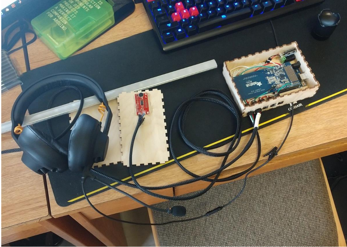
The testbench for the Arduino, I used my headphones as a speaker in order to test the microphone so that I wouldn't disturb my neighbors. The extra long cables I made make this so much easier too.
