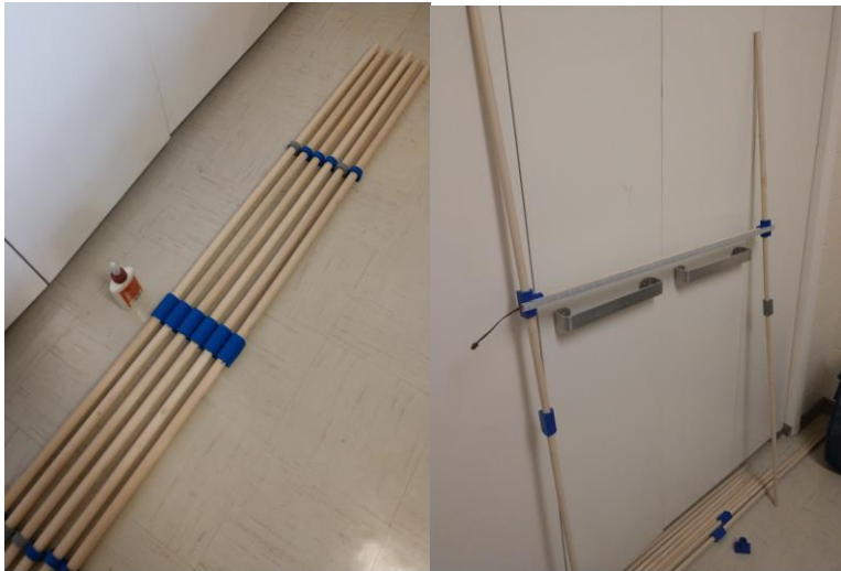
Gluing together most of the curtain masts, and the cross pieces for the LED frames in my dorm.
